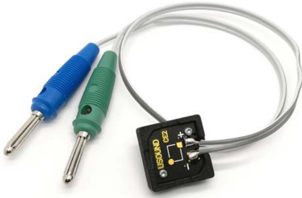
Figure 6: Positive input (BE) blue and negative input (TE) green. The colour coding matches the outputs of Amalthea.
